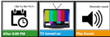
Figure 2. Exemplar composition (“If TV turned on after 8 PM, a sound clip played.”) of GaLLaG Strip
